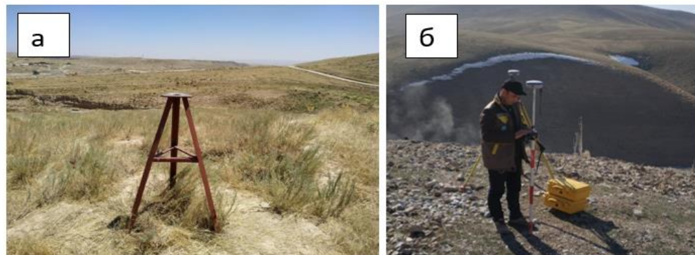
Fig. 2. Reconnaissance of geodetic points around the quarry: a - geodetic point, b - GNSS measurements
