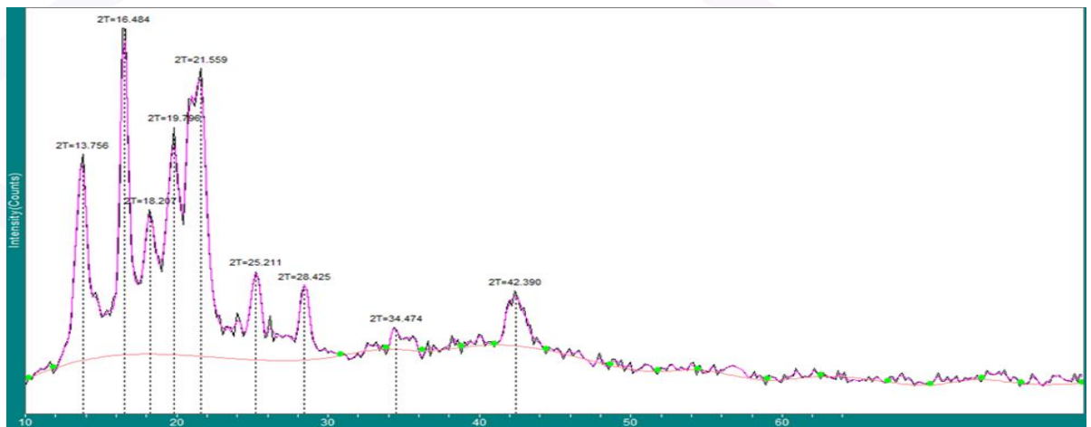
Figure (4) represents the X-ray spectrum of the matrix supported by CuSO 4 powder represents 15% at 80 C° .
